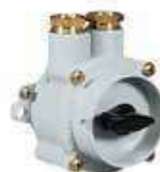
UNAV 2162 rotary two-way switch in marine grey painted brass with UNAV 1948 cable glands 250V IP66
